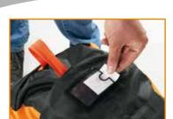
An icon allows wheel position (right/left front or right/left rear) identification
